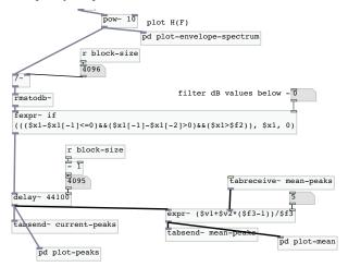
Figure 6 - Envelope peak detection mechanism.
