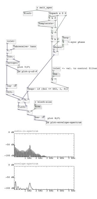
Figure 3 - The sub-patch [pd cepstrum], extracting the spectral envelope (array "envelope-spectrum") of the filtered signal (see Fig.4).
