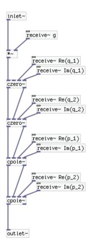
With a real filters, of course, you would just use the real versions and get rid of the imaginary patch cords. But with typical higher order audio filters, the zeros and poles will come in complex conjugate pairs, so you can expect to use the complex filters. Besides, a real number x = x + j0 anyway, so the complex ones will work in both situations.
